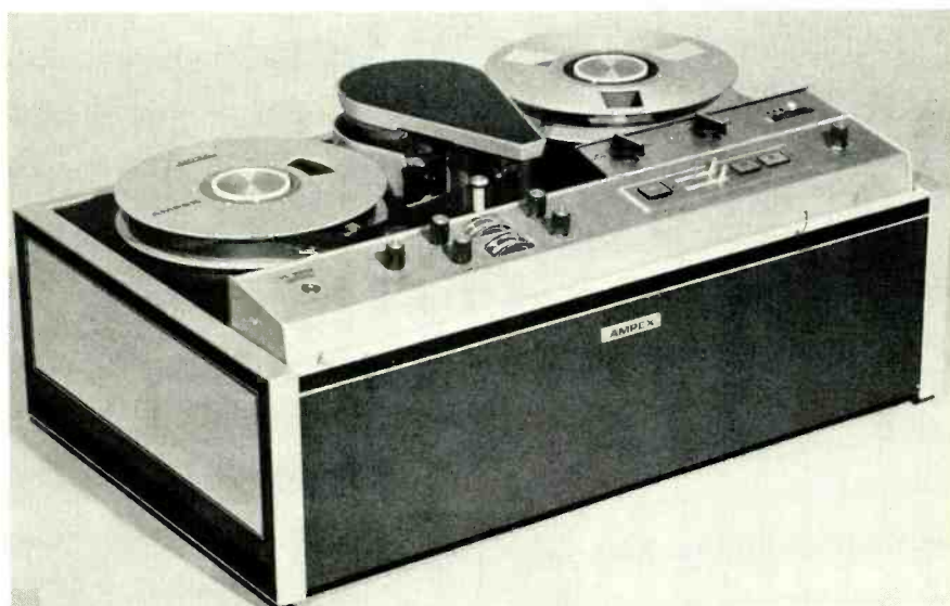
Fig. 5 Ampex's VL-7404 is the first videotape recorder designed for program logging and verification. It can log up to 38 hours of video, audio, and time information on a standard 9 \frac{3}{4} -inch reel of 1-inch tape.
